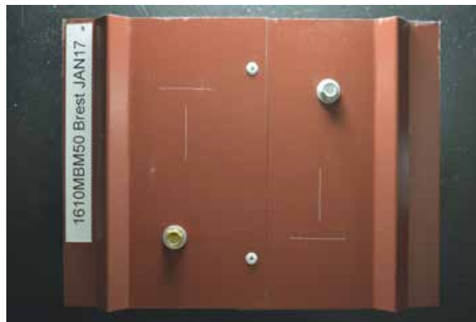
A standardised sample of Colorcoat SDP 50 for outdoor exposure testing. After 4 years, the samples were assessed. RC5+ criteria according EN 10169 were fulfilled.
