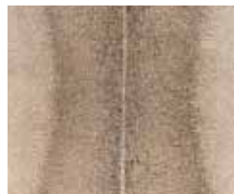
Cold-formed tube micrograph: inconsistent structure with pockets of stress and variations in mechanical properties
