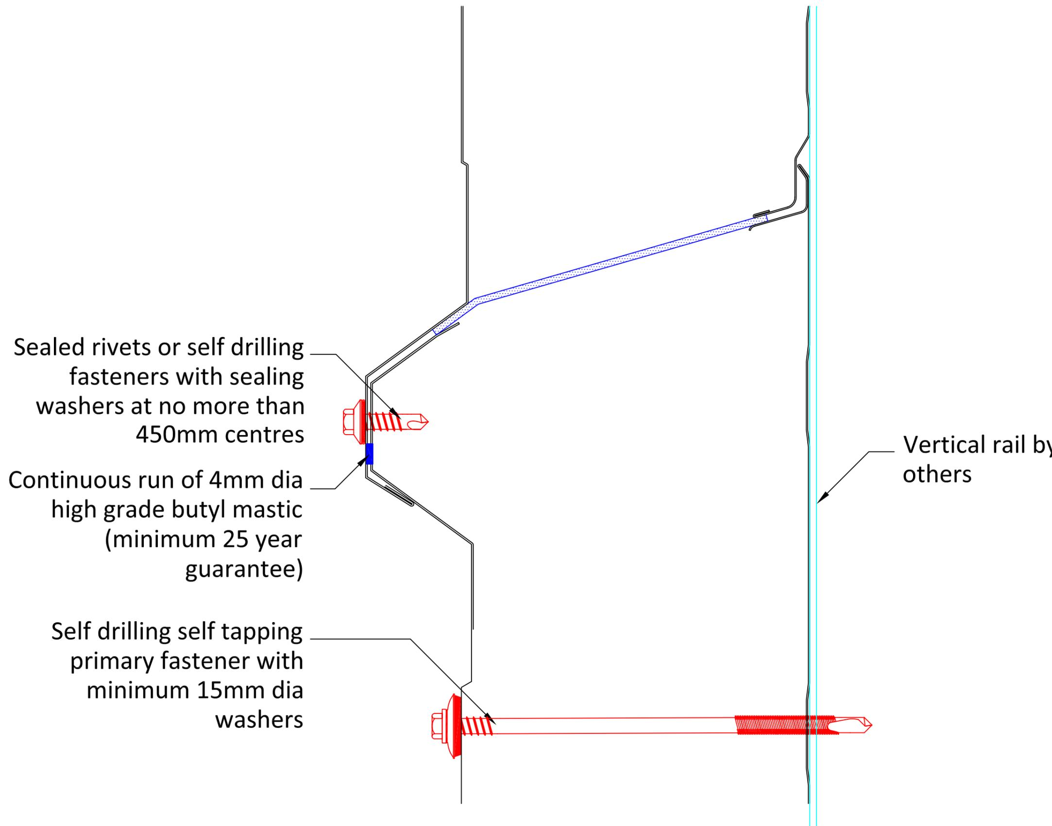
Sealed rivets or self drilling fasteners with sealing washers at no more than 450mm centres
