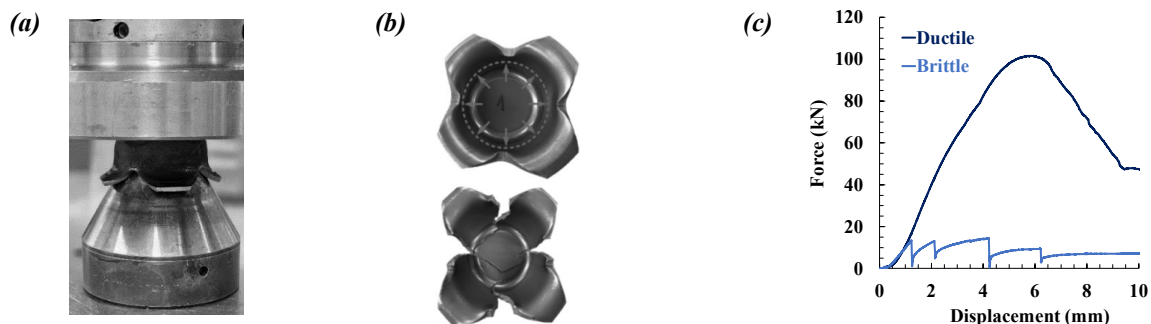
Figure 3. Images of (a) the experimental setup for the cup-opening stage of the DDC test, (b) the effect on deep-drawn cups, and (c) examples of force-displacement curves for steels with ductile and alternating ductile-brittle fracture behaviour
