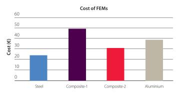
A life-cycle study of a front-end module used across a vehicle platform shows that the steel-based solution has the lowest life-cycle carbon footprint, with a significantly lower cost than either aluminium or composite plastic options.
