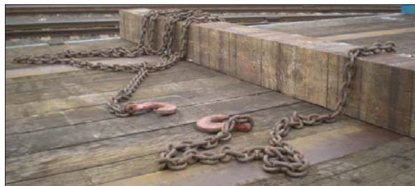
Loose chains on trailer deck can slide off.
