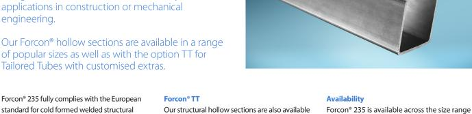
standard for cold formed welded structural hollow sections of non-alloy and fine grain steels, EN 10219. As all our tubes, they are manufactured to high quality standards and made from fully killed steel. This ensures a more uniform microstructure and makes them easier to process, offering high levels of formability and excellent weldability.
