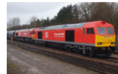
In February 2021, the UK's first locomotive powered by 100% vegetable oil pulled a 2,500-tonne load of steel coil from Llanwern to our Roundoak railhead in the West Midlands. The hydro-treated vegetable oil reduces carbon dioxide and nitrogen oxide emissions by 90% and this trial is opening the way for greater use of this fossil-free fuel alternative on the UK rail network.
